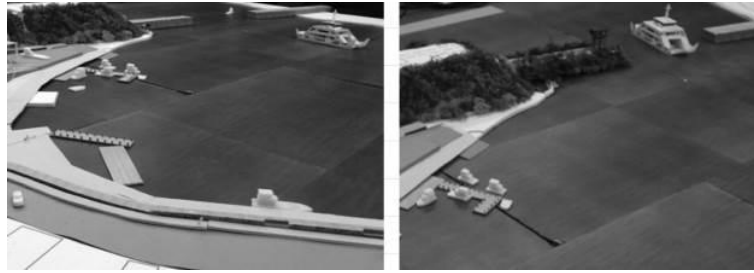
Figure 4. Model of off-shore breakwater planned by the Community Council: Model of the Naiwan area with an off-shore breakwater at the mouth of the bay. Apart from studying possible obstructions to shipping, the Council also explored ways of utilising the breakwater as tourist attraction: Its visual appearance could be improved by greenery and an observatory at its tip would allow to spot incoming ships and ferries. The model has been build by the Urban and Regional Research Institute of Waseda University.
