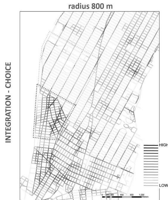
Figure 8. Manhattan - short/long segments and permeability. Segment angular analysis for combined measure of integration and choice for radius 800 meters.
