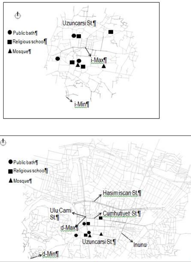
Figure 7. Comparison between axial line maps (integration R_n ) of historical city of Bursa in 1860 (top) and at present time (bottom).
