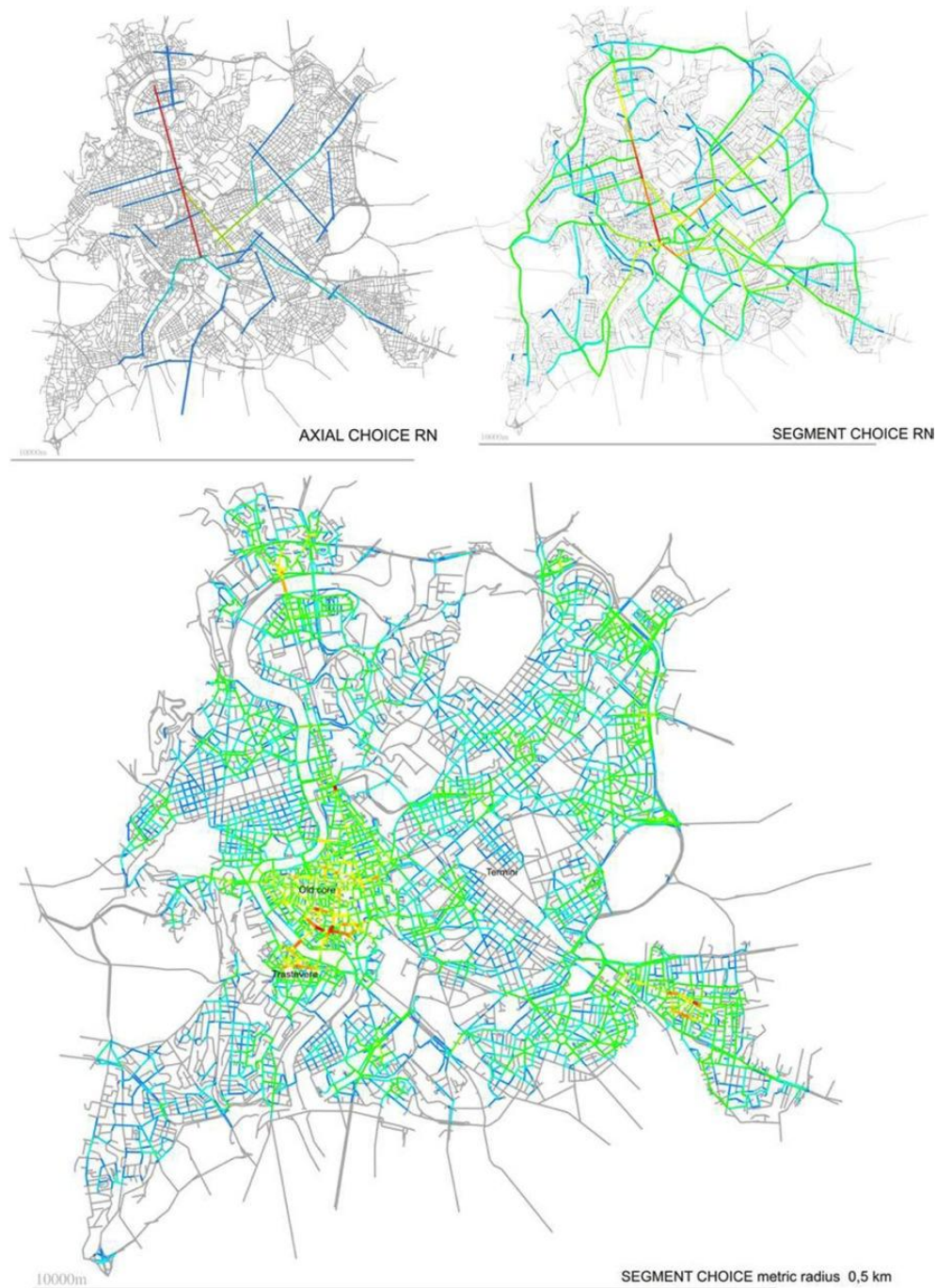
Figure 3. Route Choice system Axial and Segment modeling (Claudio Ugalde). Route from the Old Core to Trastevere is highlighted in red/yellow for 500m radius.
